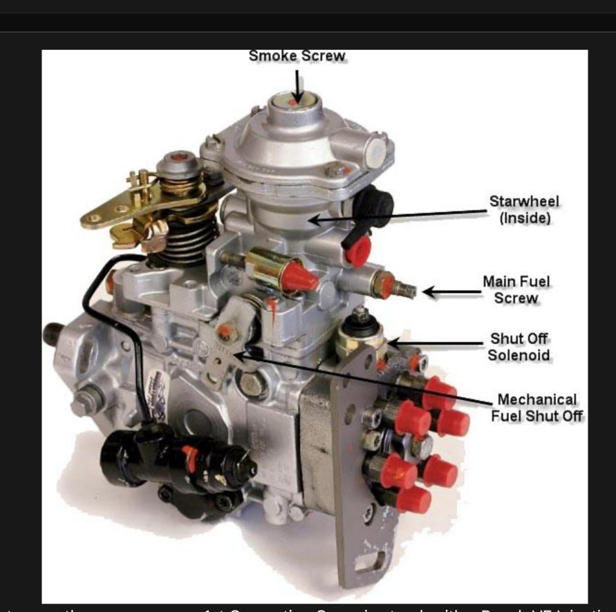
Here is a brief write up on how to turn up the power on your 1st Generation Cummins truck with a Bosch <u>VE</u> Injection pump.
