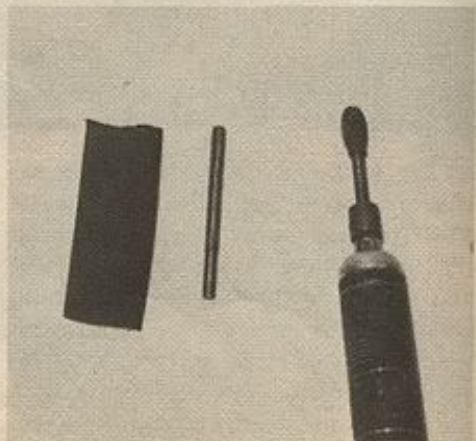
ABOVE, the tools needed are a high speed grinder, flex shaft and emery cloth.
