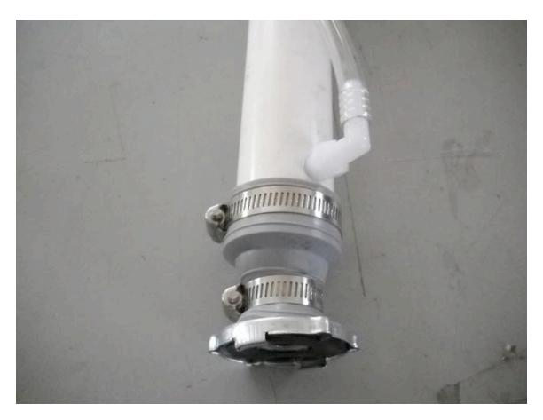
Attach the tube, and use a coathanger wire to make a clip for it what will fasten the open end to the open top of the pipe when is use. The plastic tub is important because it allows the coolant remaining in the pipe to be saved for future use instead of on the driveway. The end is simply lowered to empty the pipe's contents, if there any, into a container.
