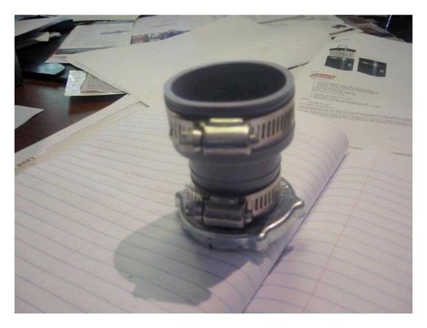
Drill and tap the PVC for the elbow 1 1/2" from the end of the pipe. Connect the adapter to the pipe.
