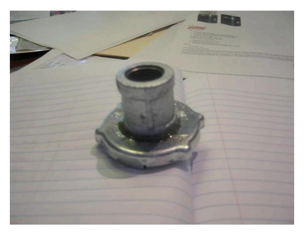
When all is ready for assembly, use clamps to tighten the small end of the adapter to the iron coupler as shown. Some RTV wouldn't hurt.
